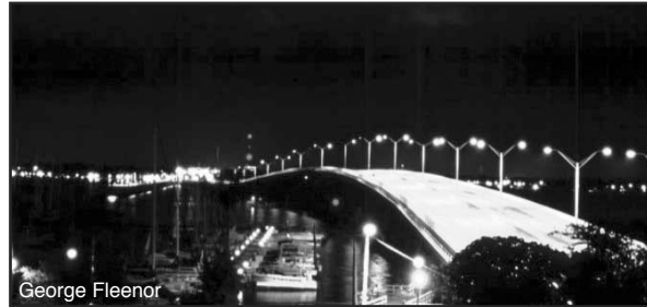
Lighting using fully shielded fixtures reduces glare and expense.
